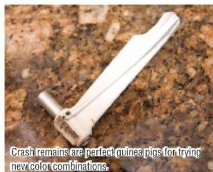
Generally, the more flexible a piece of plastic is, the harder it will be to dye.
