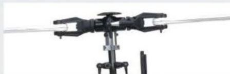
Flybarless heads are much simpler in design. The complexity is in the electronics.
