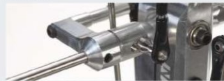
The Bell-Hiller flybar is still used today on RC helicopters. The Aurora's flybar offers some of the most precise tuning available.
