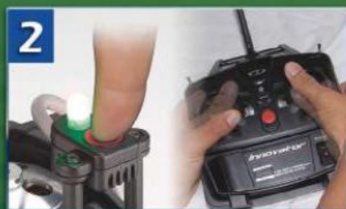
2 Calibrate max travel defined by radio gimbals
